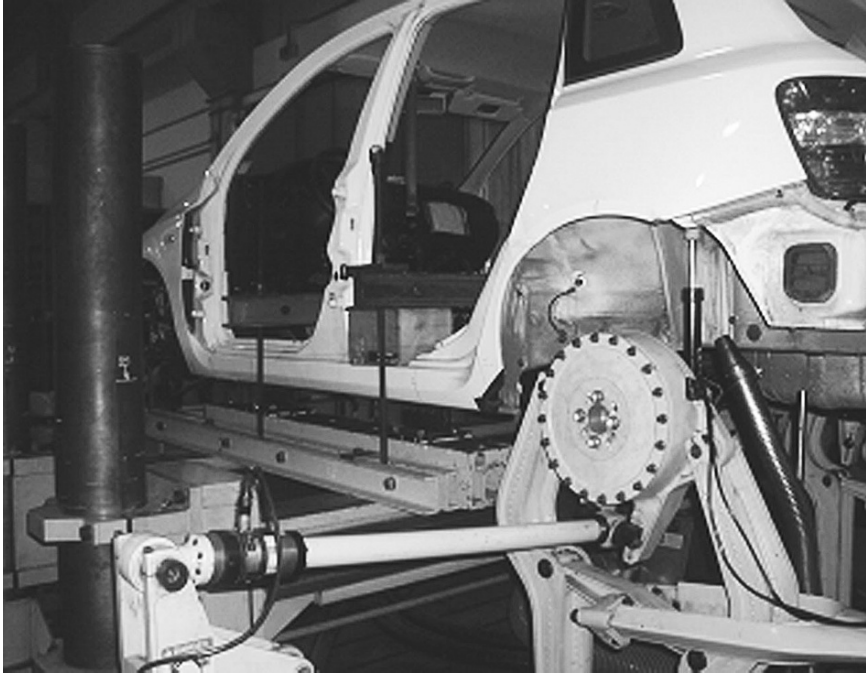
FIGURE 18.10. Fatigue test bench for a car body, complete with the most important chassis components; actuators supply rear suspension forces and torques.
