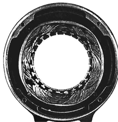
Fig. 5-19 Split-phase motor windings. (Bodine Electric Co.)
