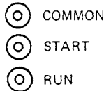
Fig. 7-45 Built-up terminals on pancake compressors manufactured before 1952. (Tecumseh)
