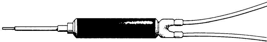
Fig. 12-6 Replacement filter drier. (Kelvinator)
