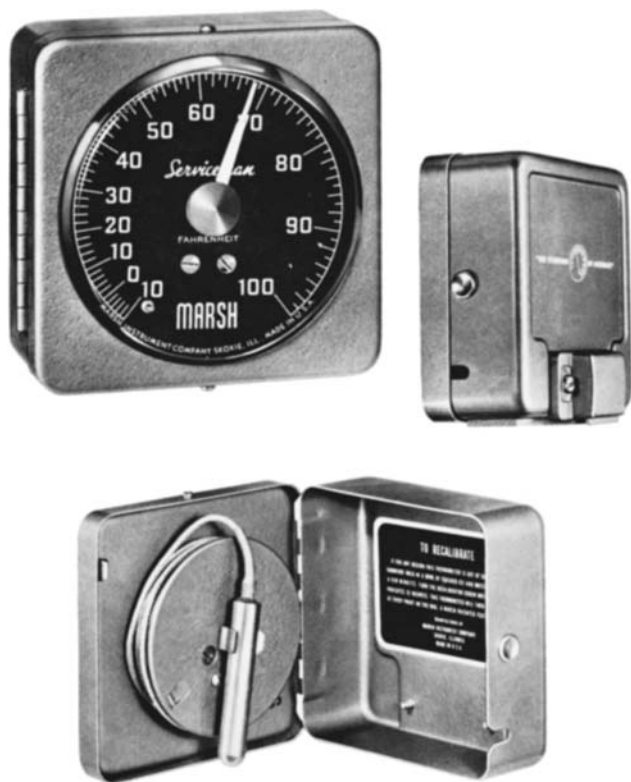
Fig. 1-30 Test thermometer. (Marsh)
