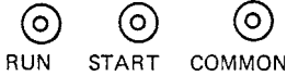
Fig. 7-43 Built-up terminals. These are on the obsolete twin-cylinder internal mount H models. (Tecumseh)
