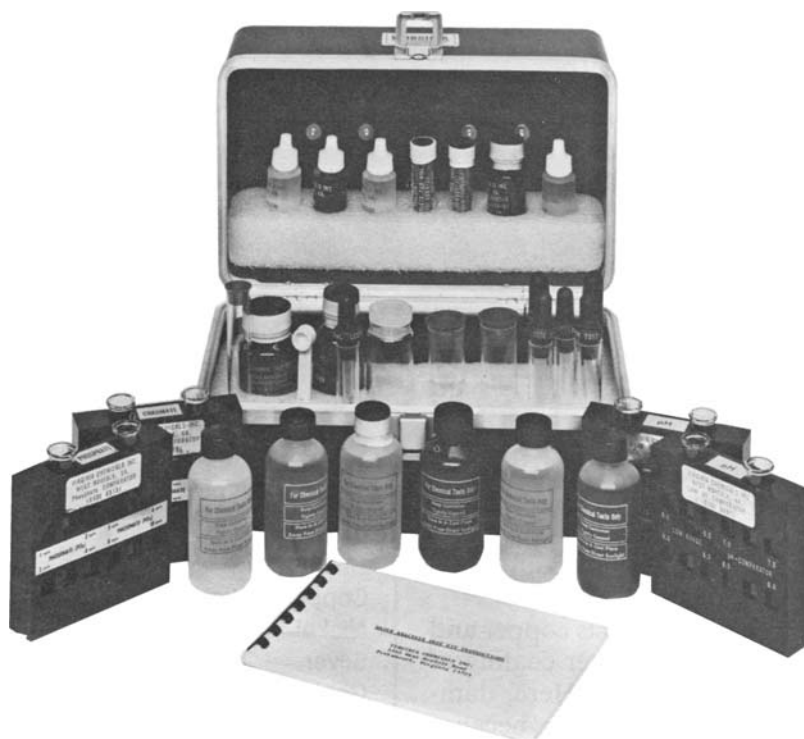
Fig. 9-1 Field kit for testing pH, phosphate, chromate, total hardness, calcium hardness, alkalinity, and chloride. (Virginia Chemicals)
