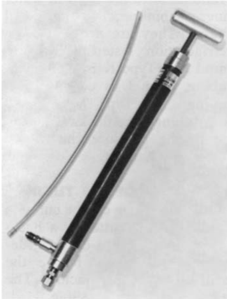
Fig. 1-59 Oil changing pump. (Thermal Engineering)
