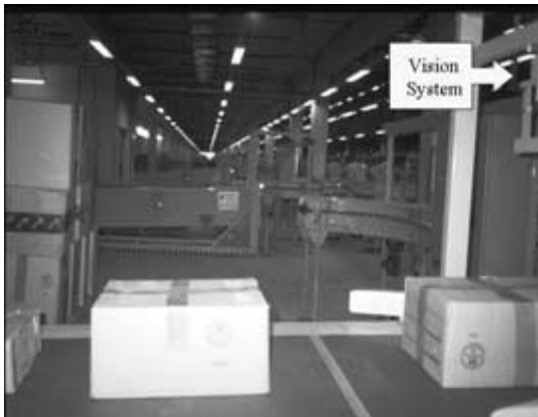
FIGURE 9-19 Vision system used in automated receiving inspection.
