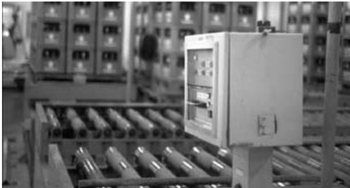
FIGURE 7-44 Smart card reader for driver-load-vehicle verification.
