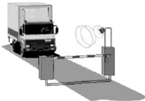
FIGURE 9-16 RF tag application in yard management.
