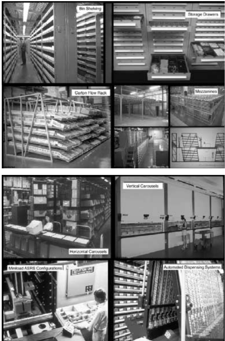
FIGURE 8-26 Small item storage systems.
