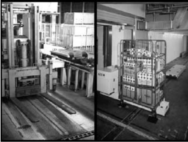
FIGURE 8-41 Automated, direct vehicle loading.
